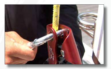
Easy to use, it is used on a free halyard, or a spare line that is hoisted with the mast ladder.
